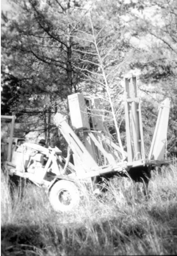
Figure 9.3. Tree spade used for planting large saplings or small trees. Photo courtesy of Dr. Schilling, Louisiana State University School of Forestry.
